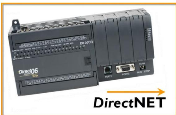
For example, some AutomationDirect PLCs use a serial RS-232C or RS-422 physical layer network with the DirectNET protocol for communications. This protocol can be used for PLC-to-PLC communication over a point-to-point or multipoint network using standard PLC instructions, or to talk to AutomationDirect's C-more HMIs.
