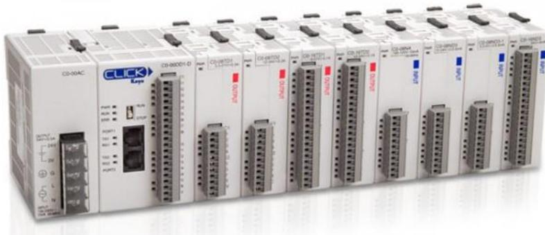
Another option with PLC hardware is the modular base configuration. With this style of PLC, a separate base unit that holds the modular components is needed. Each module will seat into a slot on the base unit that is used to connect the module to the backplane already installed in the base. These bases come with different numbers of slots and some with power supplies built in. Typically, the first two leftmost slots are dedicated for the power supply and CPU.
