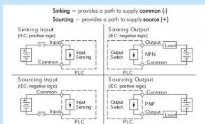
Make the right choice the first time when selecting the type of I/O points for your application by reviewing these sinking and sourcing concepts.
