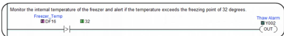
Ladder Logic is the most widely used programming language in industrial automation today. Its ease of use, traceability, and visual representation of physical components make it the favored programming method of many engineers. If you are new to PLC programming and would like to try Ladder Logic for yourself, download any of our programming software packages mentioned below for free and see what you think. After all, experience is the best teacher.
