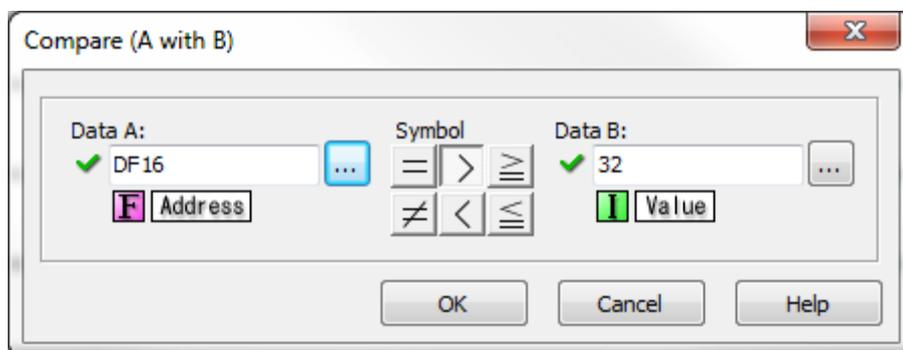
The Compare contact dialog box allows us to select any of the six different comparison methods. For this example, we have selected Greater Than so that if our Freezer Temperature ever becomes Greater Than the number 32, our Compare contact will become true.
